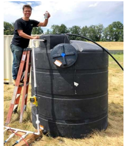
Figure 34 Fulton Schools Associate Professor Leon van Paassen takes samples of extracted water at the site of the project to test microbially induced desaturation for mitigating
